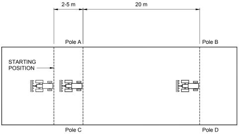
Figure 3 – Measurement of Operating Speed for Tractor-drawn Weeder
