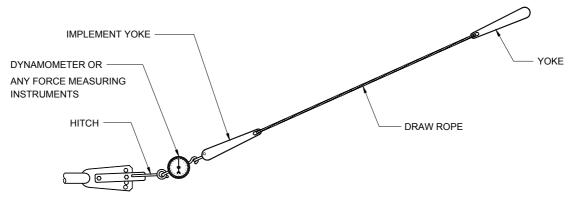
Figure 4 – Draft Measurement for Animal-Drawn Weeder
