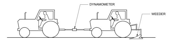
Figure 6 – Draft Measurement for Tractor-Drawn Weeder
