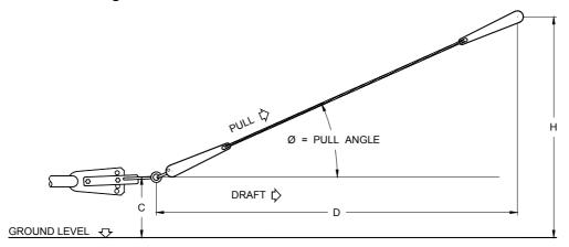
Figure 5 – Angle of Pull Measurement for Animal-drawn Weeder
