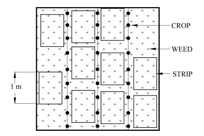
Figure 4 – Marked Strip for Assessment of Weeding Efficiency
