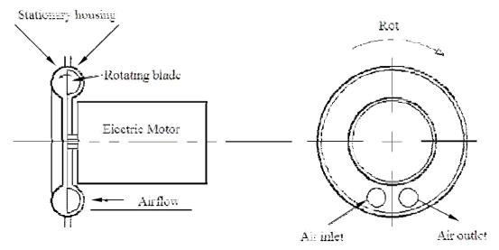
Figure 21a. Vortex blower rotating in right half of the torus-shaped housing. (Fan Handbook Selection, Application and Design by Frank P. Bleier)
