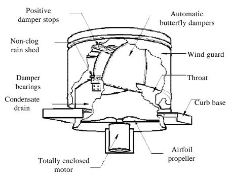
Figure 19. Parts of a roof ventilator. (Fan Handbook Selection, Application and Design by Frank P. Bleier)
