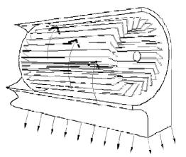
Figure 20. Direction of air flow in cross-flow blower. (Fan Handbook Selection, Application and Design by Frank P. Bleier)
