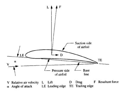
Figure 1. Free Body Diagram of Airfoil Blade (Fan Handbook Selection, Application and Design by Frank P. Bleier)
