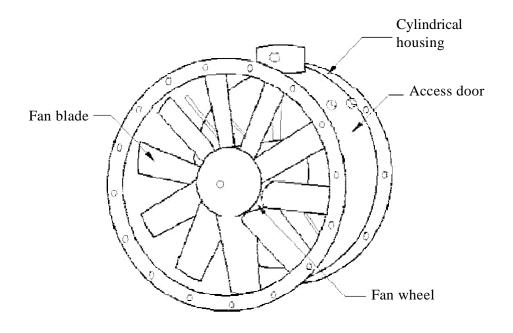
Figure 9. Parts of tube-axial fan with cylindrical housing. (Fan Handbook Selection, Application and Design by Frank P. Bleier)
