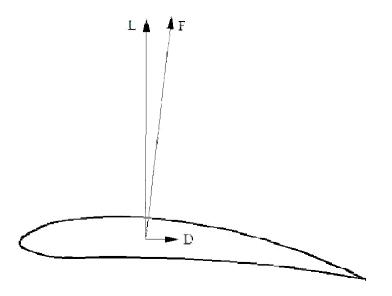
Figure 2. Lift and drag on fan/blower blade. (Fan Handbook Selection, Application and Design by Frank P. Bleier)
