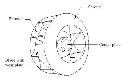
Figure 16. Parts of centrifugal fan with radial tip blades. (Fan Handbook Selection, Application and Design by Frank P. Bleier)
