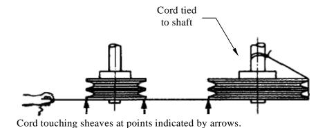
Figure 23. Use of a chord to check the alignment of the sheaves. (Fan Handbook Selection, Application and Design by Frank P.Bleier)
