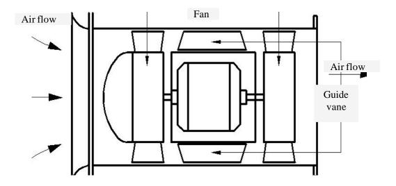
Figure 11a. Two-stage axial-flow fan rotating at the same direction. (Fan Handbook Selection, Application and Design by Frank P.Bleier)
