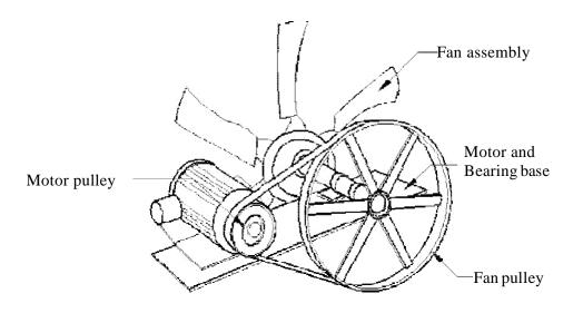
Figure 3. Parts of belt-driven propeller fan/blower (Fan Handbook Selection, Application and Design by Frank P. Bleier)
