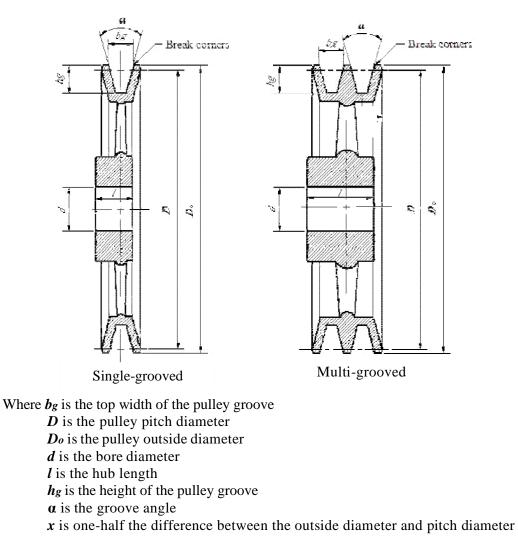
Figure 25. Types and designation of dimensions of V-pulleys
