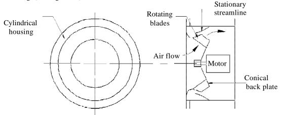
Figure 18. Fan wheel with conical back plate. (Fan Handbook Selection, Application and Design by Frank P. Bleier)
