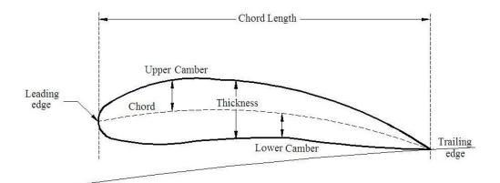
Figure 7. Parts of asymmetric airfoil blade. (Wikipedia, Airfoil)
